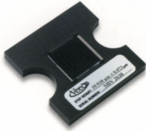
10 Micron Step Height Standard
