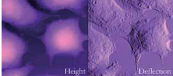
Mouse Fibroblast L-cell. Scan size 60 \mu\text{m} x 60 \mu\text{m} and Z-scale = 13 \mu\text{m} . Cells courtesy of Nate Bouxsein and Professor Cyrus Safinya, USCB, CA
