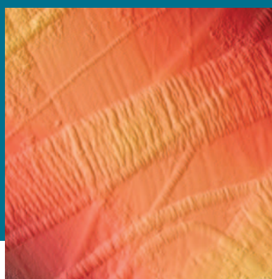
Native Collagen fibrils exhibiting the typical 67nm banding pattern. 8.5 \mu m scan.
