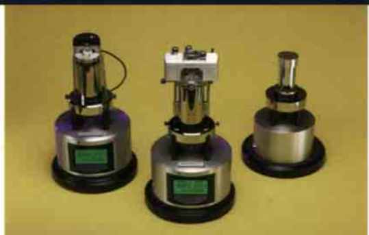
The MultiMode with the SECPM head (left); the MultiMode with the ECAFM head (middle); and ECSTM (right).
