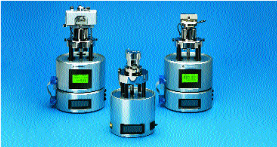
Figure 1. From left to right: Digital Instruments MultiMode SPM platform configured for Electrochemical AFM; an ECM platform configured for Electrochemical STM; an LFM platform configured for SECPM. Other configurations look nearly identical to one of these three.
