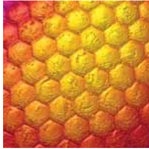
A three-dimensional profile of a multifaceted insect eye . Optical profiling reveals high detail of complex life science organisms with a completely non-contact, damage-free measurement. 309µm x 235µm FOV.
