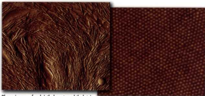
Height of polystyrene-b-polyvinylpyridine in methanol. 1µm scan.
