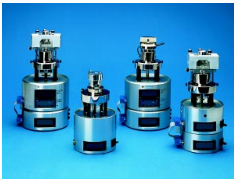
The NanoScope® EC SPMs (from left to right): MultiMode™ EC AFM, EC STM, MultiMode EC STM, and Contact EC AFM, each with their respective electrochemical fluid cells.
